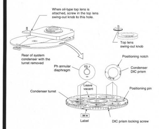
5 Apply labels to the side of the turret in accordance with the DIC prisms and Ph annular diaphragms that were installed. Apply each label in the position that appears in the front when the system condenser is mounted on the microscope and the DIC prism or Ph annular diaphragm in question is inserted into the optical path. (The label will be on the diagonal from the DIC prism or Ph annular diaphragm in question.) Place the label "A" on spaces for vacant holes.
