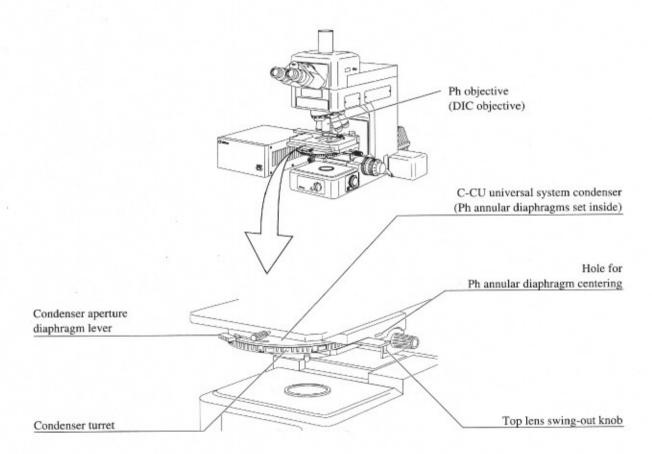
(Ph microscopy cannot be performed when using an oil-type top lens.)
