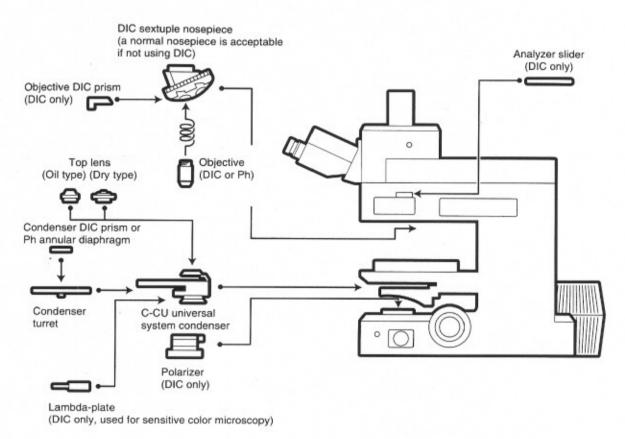
DIC only: Components needed only when performing DIC microscopy.
