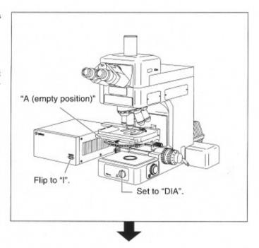
Place the specimen on the stage, and focus on the specimen with the 10× Ph objective (Ph1).
