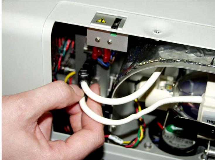
**Tip:** the 2-pin lamp power connector will only attach in the correct orientation. If you are having difficulty attaching the connector, try rotating it by 180°
