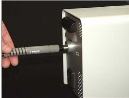
**Tip:** When the light guide is fully inserted, the line on the light guide insertion label will be right up against the light guide port.
