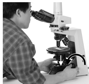
Then look into the eyepieces and lower the stage.
