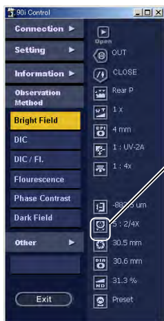
Condenser module controls display button
