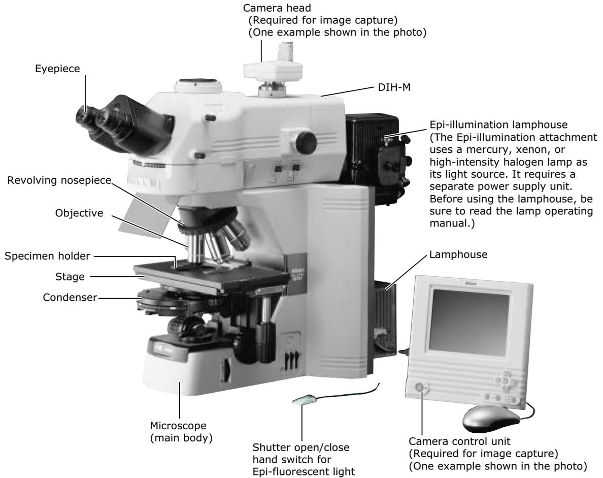
3.2 Names of Parts Used to Make Adjustments
