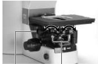
Focus the condenser using the condenser focus knob.
