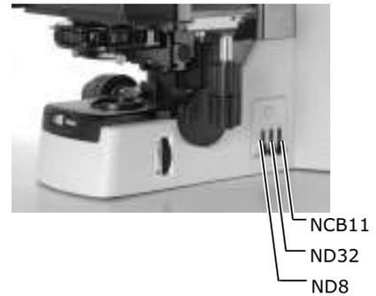
**4** Push in the optical path switching lever to direct the full optical path toward the binocular section.
