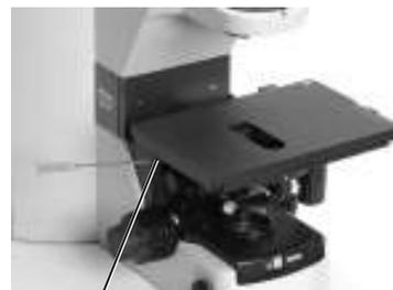
Fixing the stage with centering function
