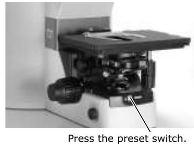
**3** Move the ND8, ND32, and NCB11 filters into the optical path.
