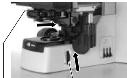
Fully open the aperture diaphragm using the aperture diaphragm lever.
