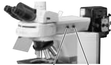
Fully open the field diaphragm. Fully open the aperture diaphragm.
