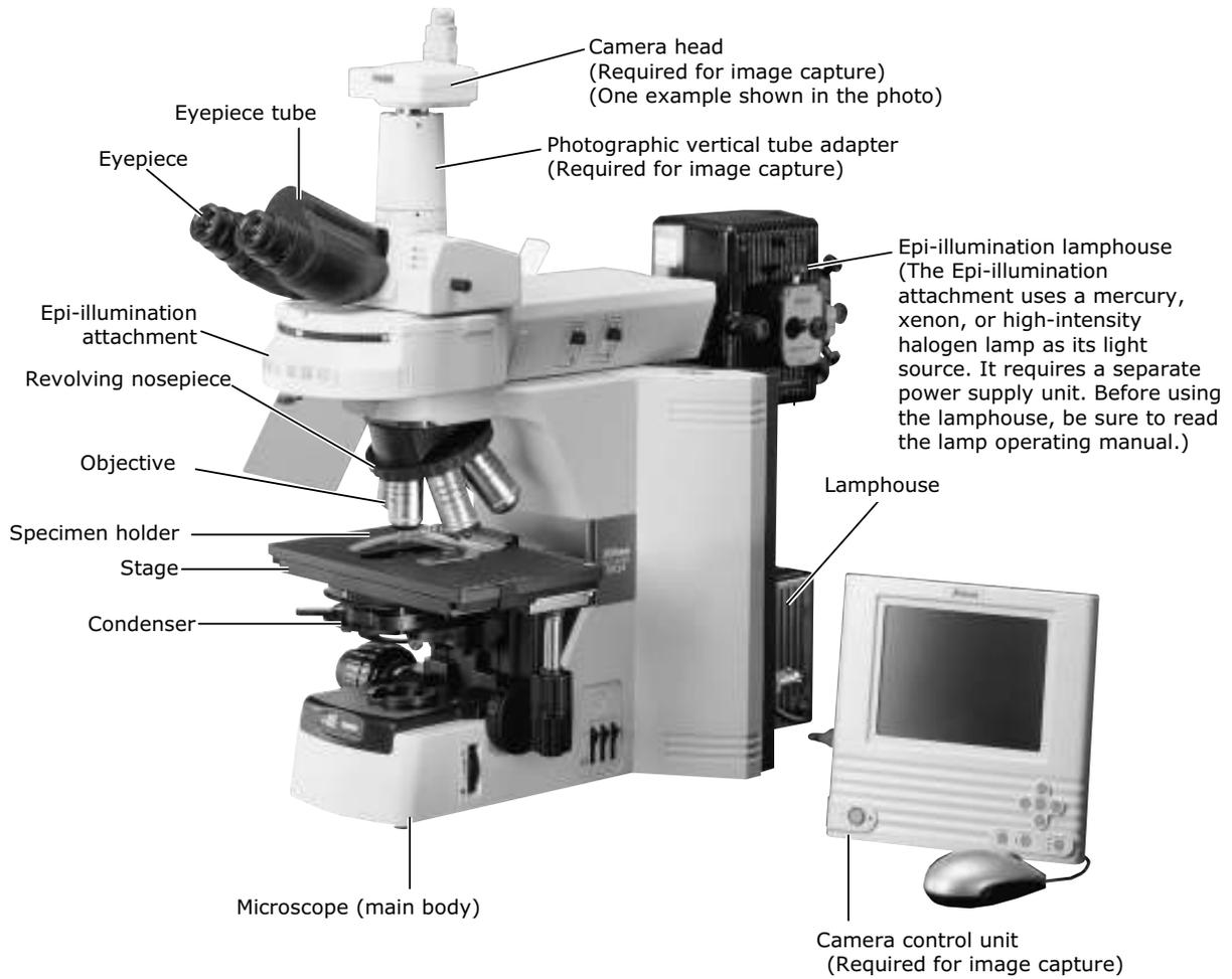
2.2 Names of Parts Used to Make Adjustments
