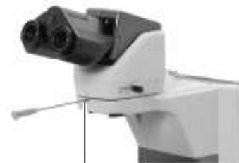
Fixing the eyepiece tube
