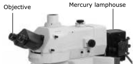
**(11)** Attach the eyepiece by aligning the projection of the eyepiece tube sleeve with the notch at the objective.
