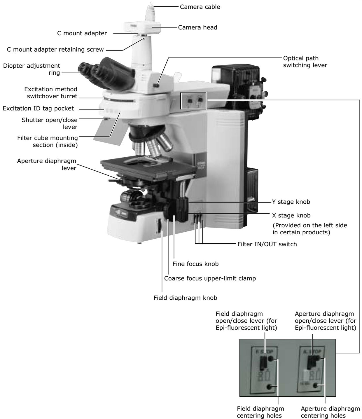
2.2 Names of Parts Used to Make Adjustments
