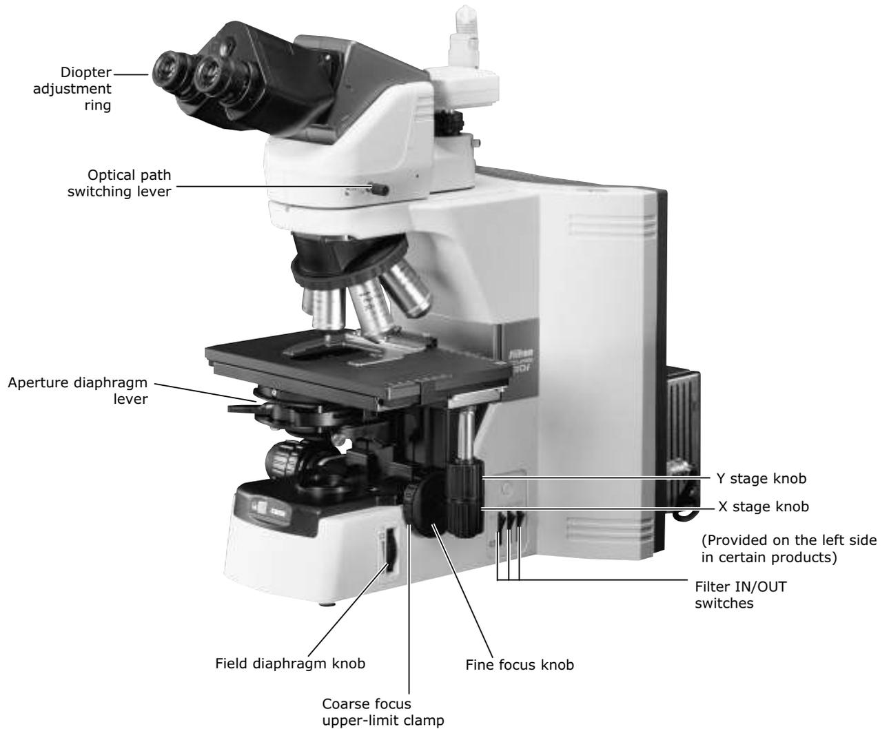
1.2 Names of Parts Used to Make Adjustments
