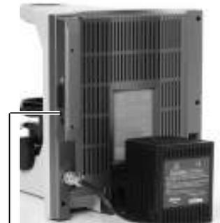
**(10)** Attach the mercury lamphouse to the back of the bayonet mount. (For more information, refer to the instruction manual provided with the super high-pressure mercury lamp power supply.)
