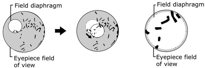
**12** Switch to the desired objective and view the specimen. Adjust the field diaphragm and aperture diaphragm each time you change objectives.
