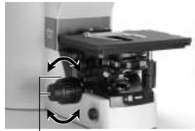
Focus on the specimen using the coarse and fine focus knobs.
