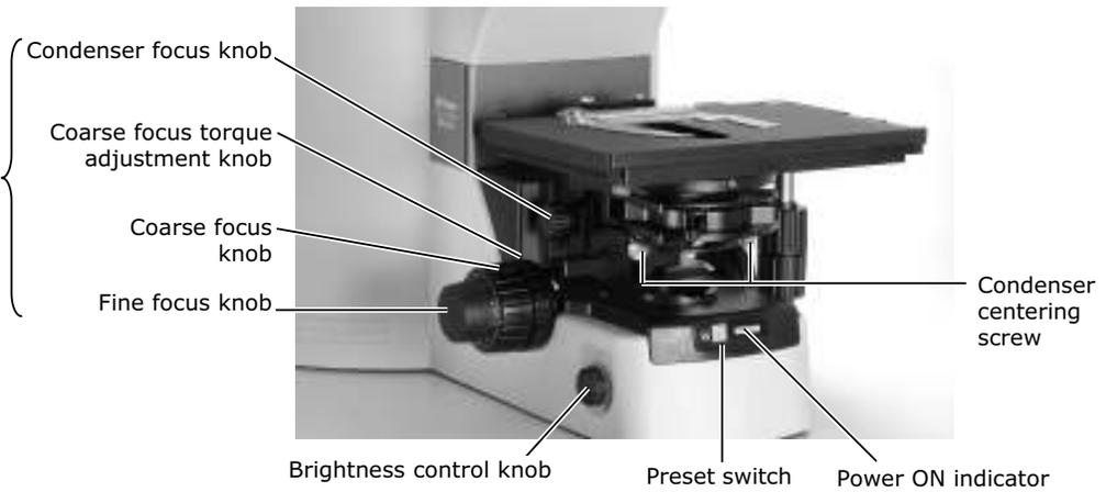
3.2 Names of Parts Used to Make Adjustments
