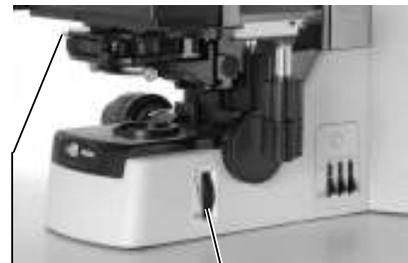
Aperture diaphragm lever Field diaphragm knob
